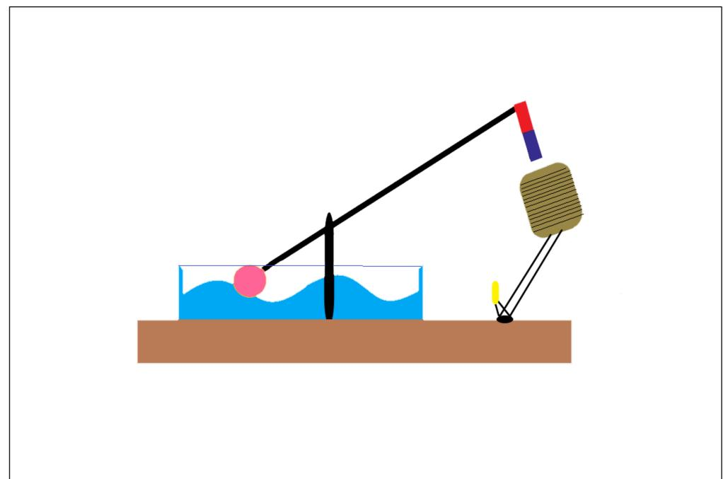
The energy of the waves is converted into kinetic energy of the magnet and then into electrical energy in the coil, which lights up a LED or charges a capacitor.
