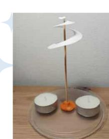
Rising warm air can power turbine. Conversion of thermal energy into mechanical energy. Support active research in class, experiments, conclusion building, theory explanation.
