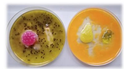
In this case, the aim of the experiment is to determine whether the gummy candy contains gelatin or agar. This is done either by means of catalases present in certain fruits or by means of the Biuret reaction.
