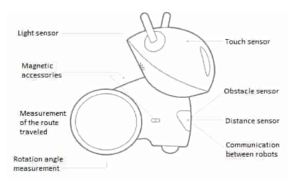
The robot has many built-in sensors to help you learn and play. These sensors and enclosed inside the housing.
