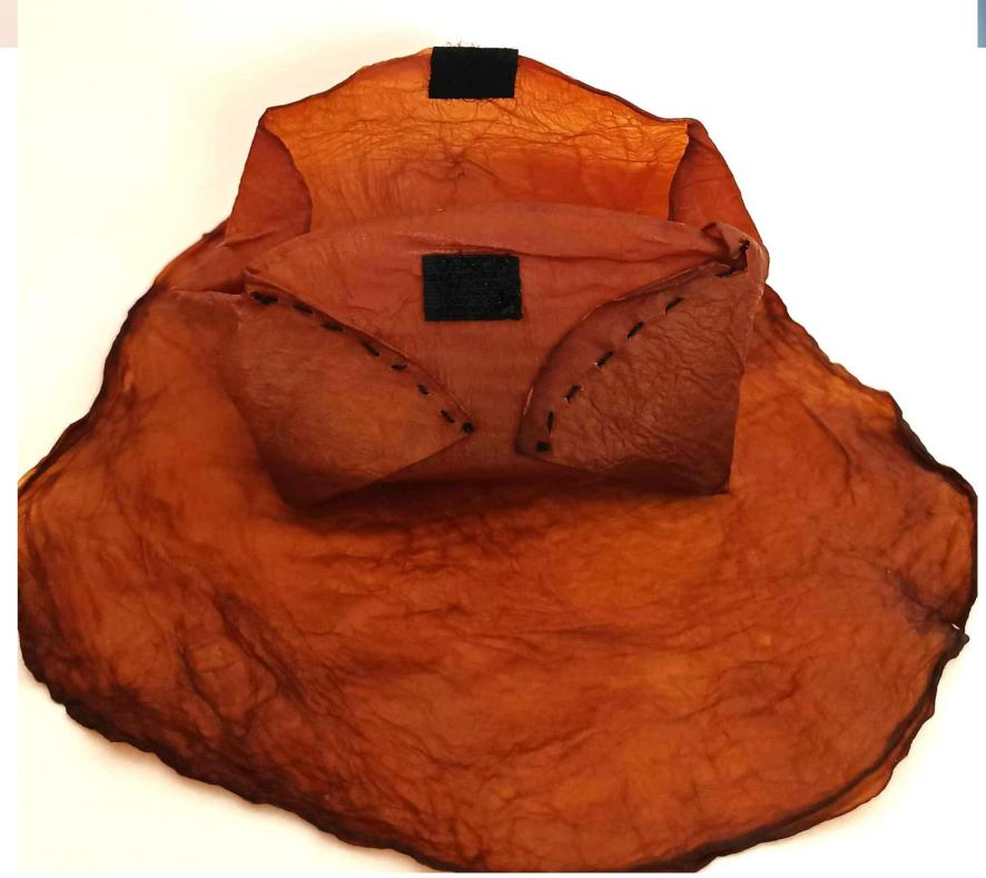
The photos show the packaging that we managed to create. The material can be sewn with thread. We created packaging for a bank card and a case for headphones.
