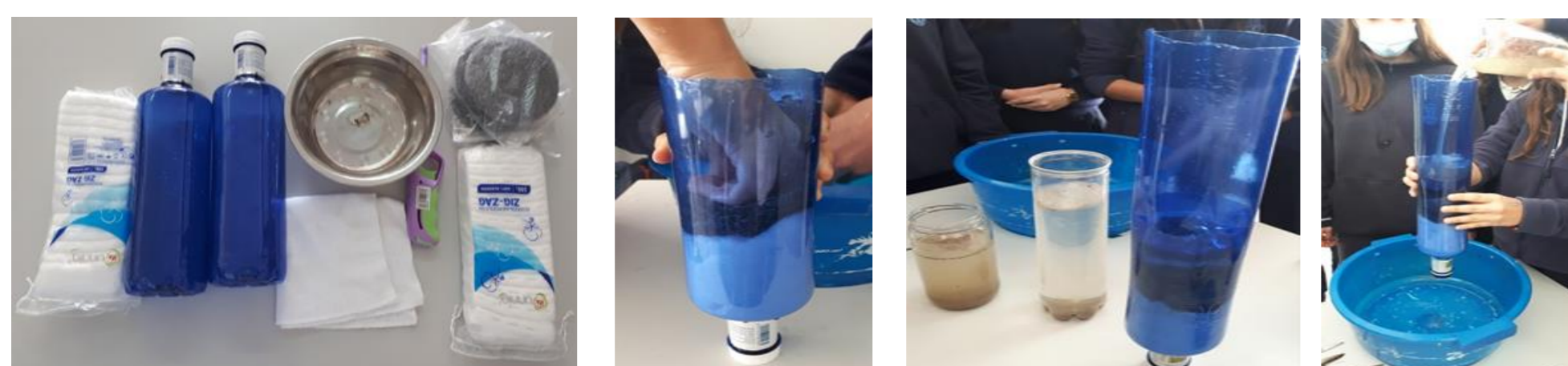
The particles of arsenic bind to iron hydroxide, and the resulting molecules are filtered through the cotton layer.
