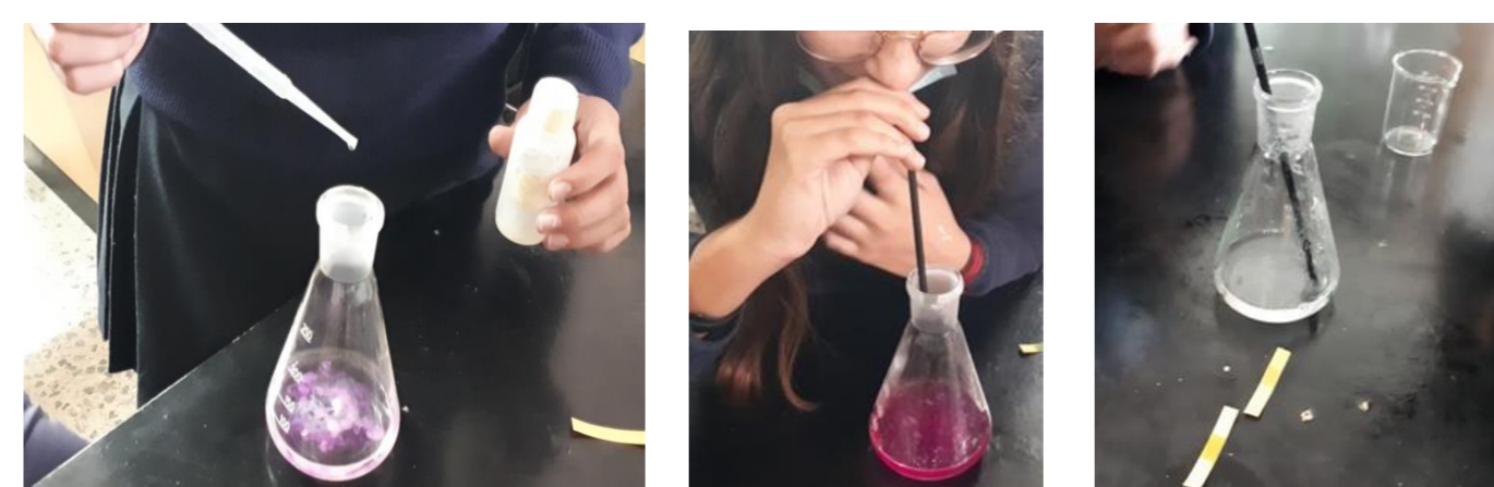
Decreasing the pH of seawater with phenolphthalein by absorption of CO 2
