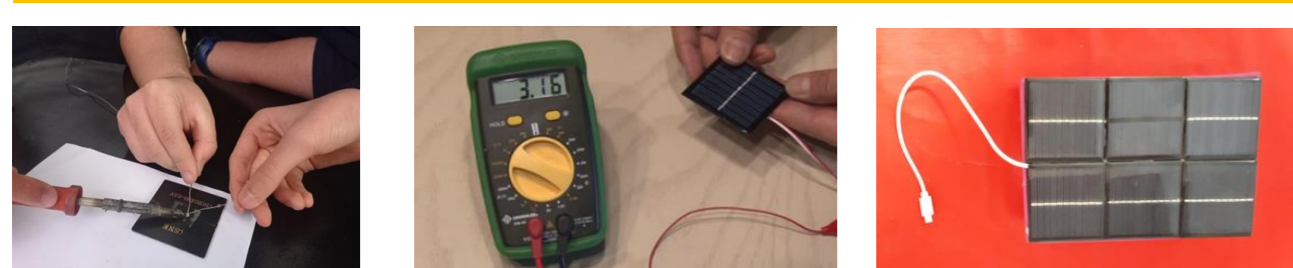
Components: a small solar cell, a standard diode and a cable with USB port.
