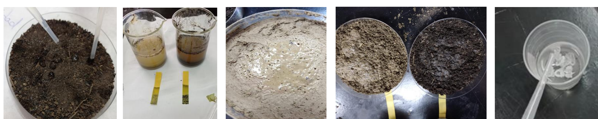
Hydrophobicity, pH comparative, presence of organic matter, presence of carbonates and detection of microbial activity.
