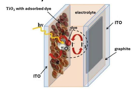
Their construction incorporates several key materials like electrically conducting glasses (ITO), titanium dioxide (TiO<sub>2</sub>), graphite, and natural dyes obtained from fruits and flowers like raspberries or rose petals.
