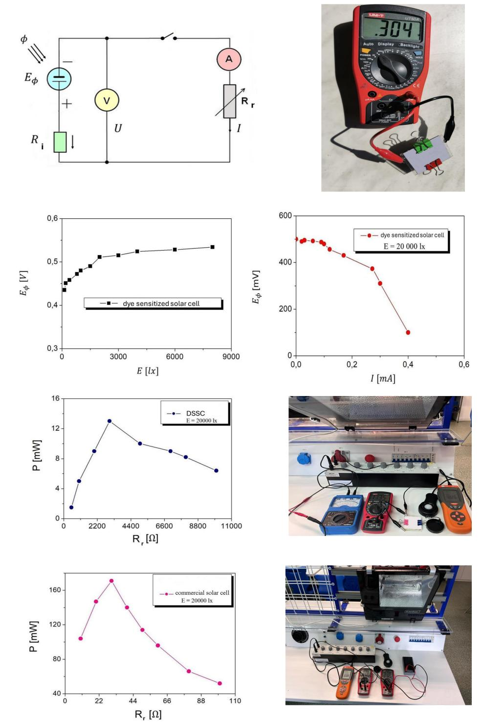
It was possible to determine the optimal load parameters for standard photovoltaic cells and DSSCs at which maximum power is transferred to the receiver. The research showed that the parameters and properties of the measured systems depend on light intensity.
